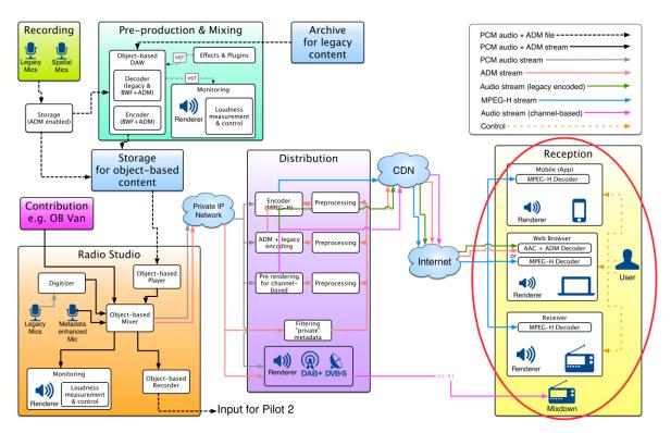
Figure 1: Reception stage in the global architecture
