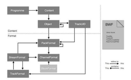
Figure 5: Diagram of the Audio Definition Model
