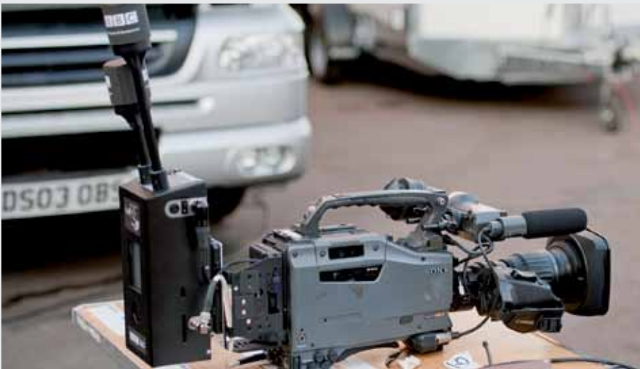
Figure 1: transmitter of the halfRF system attached to the rear of a broadcast camera
