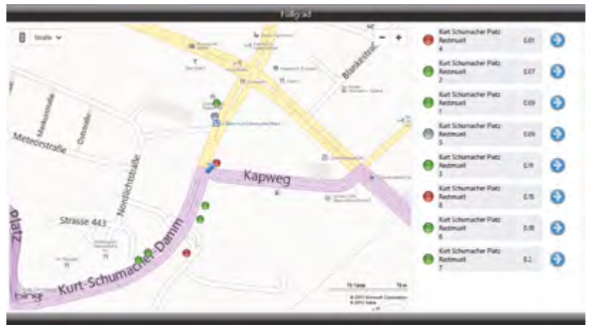
Figure 3: Mobile fill-level application
